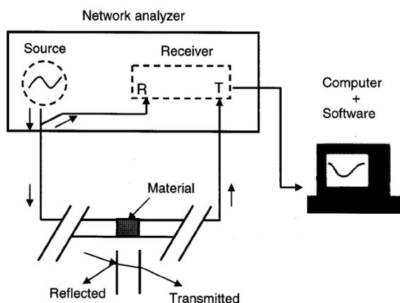
**Fig. 1. Schematic of a transmission line – waveguide method**
